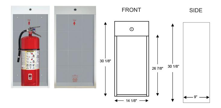
National Fire's Classic series are surface mounted cabinets that are both practical and economical. Theft and vandal resistant; these cabinets remain locked at all times, allowing emergency access through means of breaking the scored acrylic glass. Cabinets come complete with scored acrylic, breaker bar, key and decal (English & French). Perfect for parking garages, warehouses, industrial areas and construction sites.
