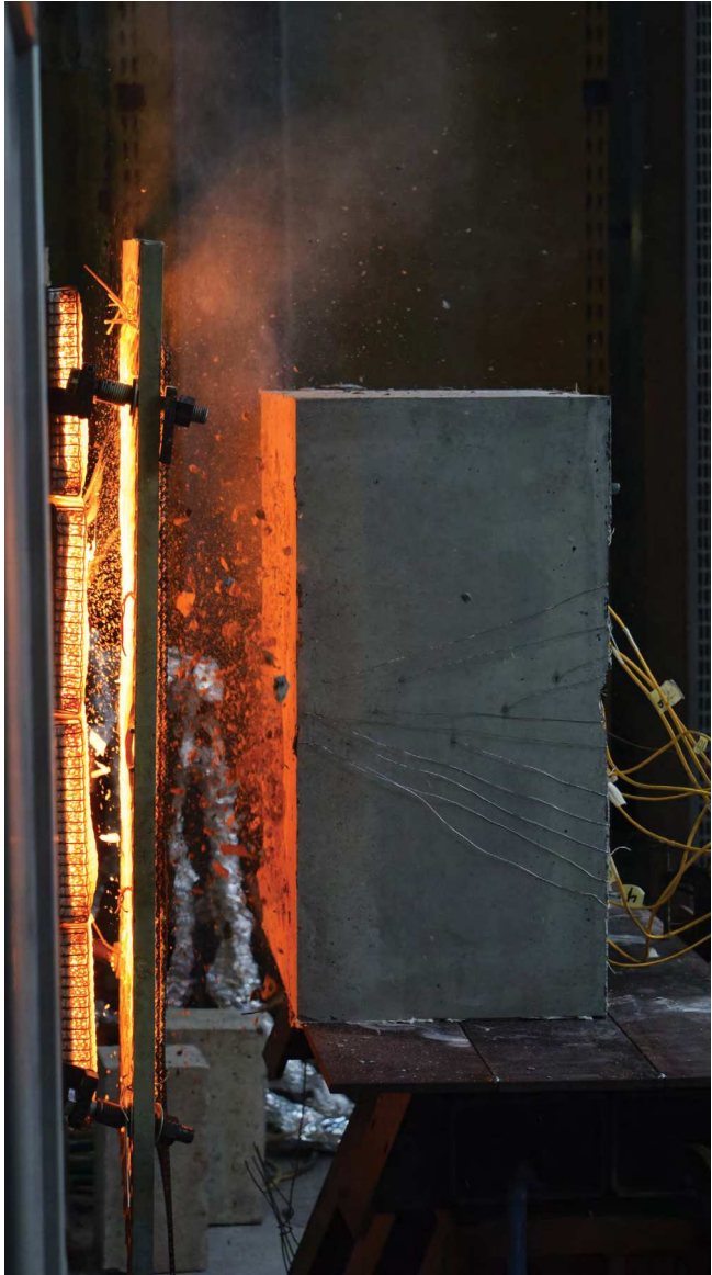
Concrete spalling in UQ’s Heat-Transfer Rate Inducing System (H-TRIS) test apparatus.
